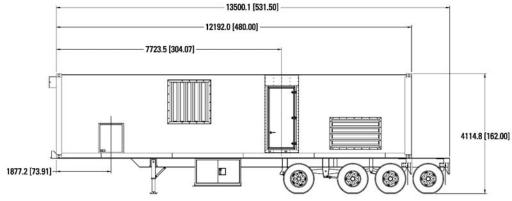
The power module must have support under the center when set on the ground.
